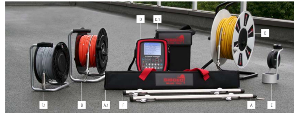
A Digital inclinometer probe A.1 Travel bag for both inclinometer and dummy probes B Light inclinometer cable reel C Heavy-Duty cable D Archimede readout D.1 Archimede carrying case E Pulley assembly F Dummy probe F.1 Cable for dummy probe
