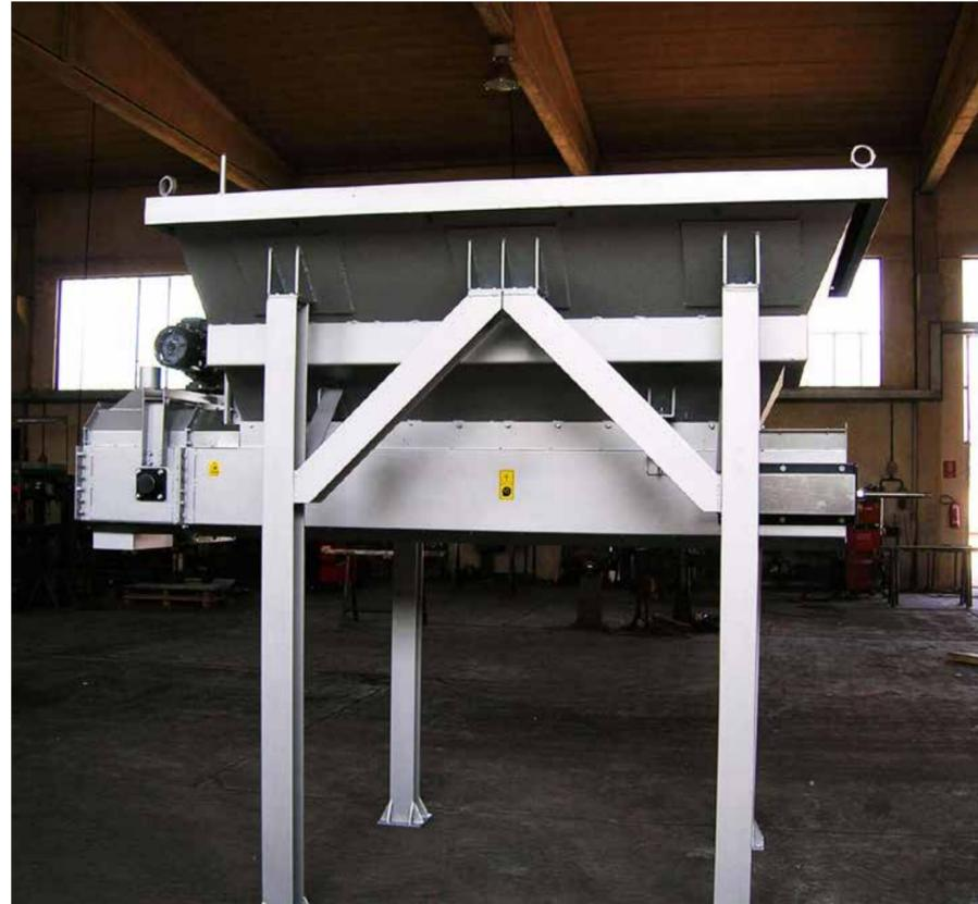
↑ Loading hopper composed of conveyor belt with weight detection
