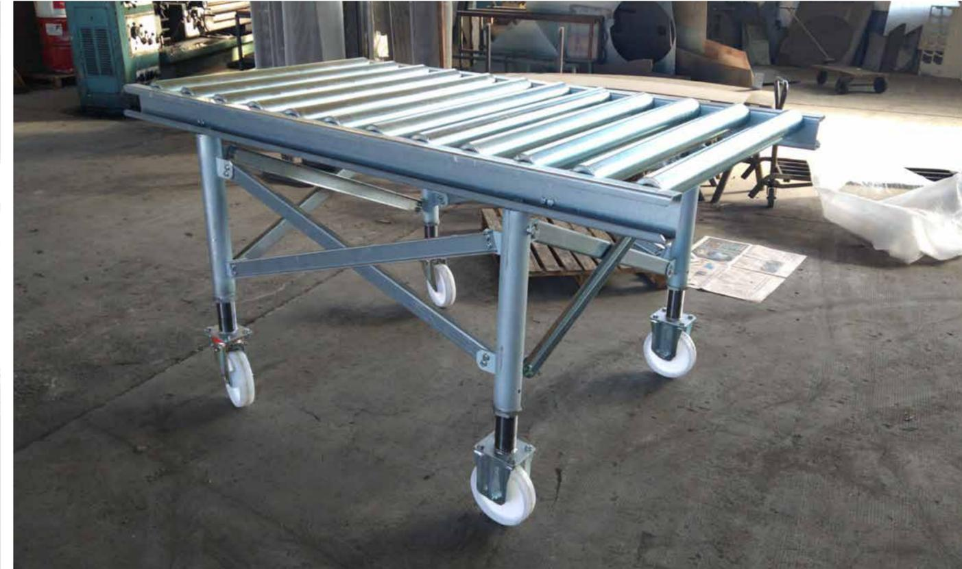
↑ Calibrate roller conveyor for work bench extension
