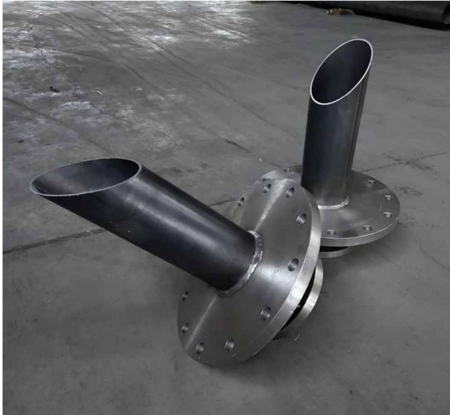
↑ Reductions for pump tank connections
