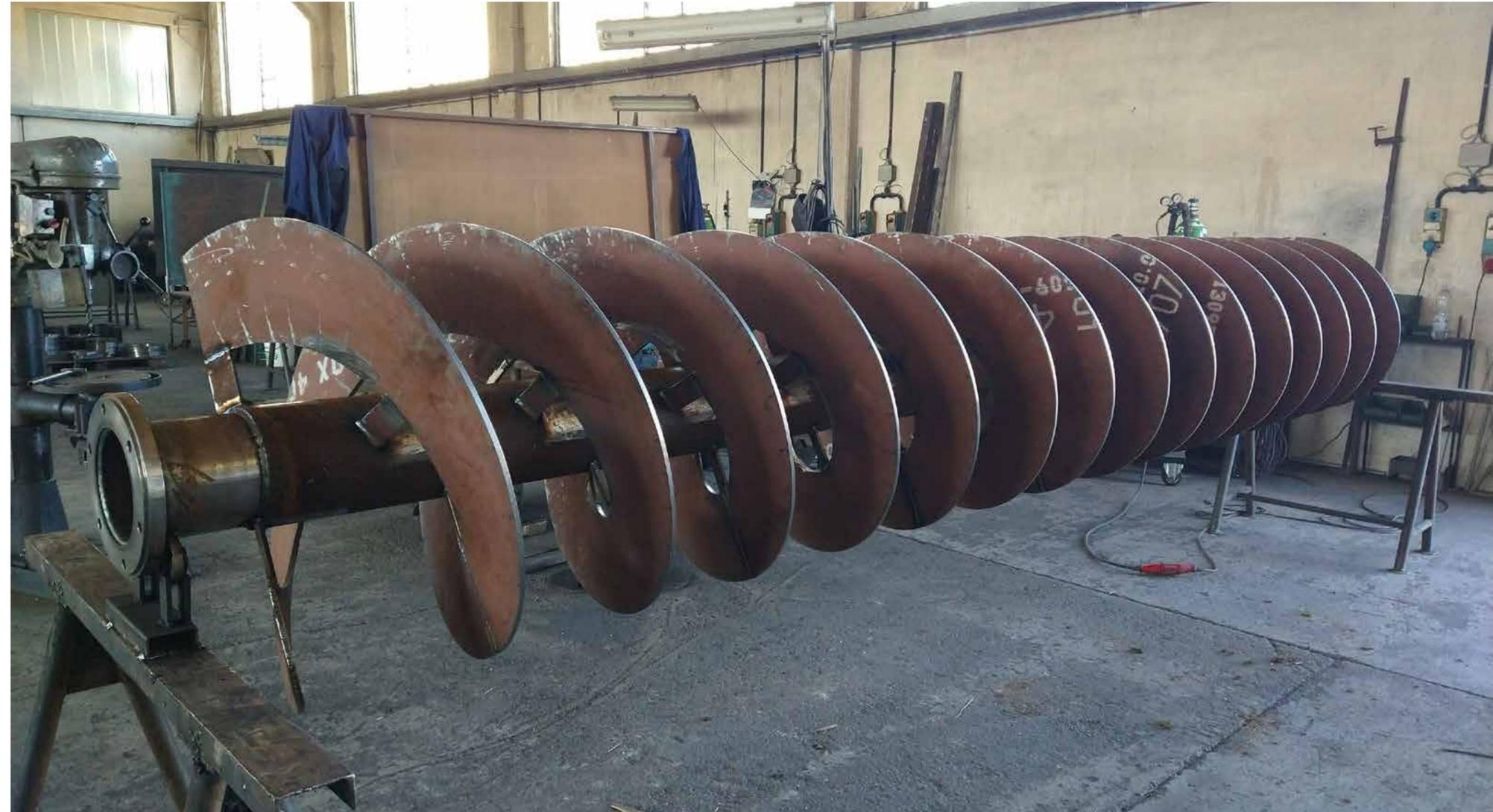
↑ Anti-wear auger for sediment deposition
